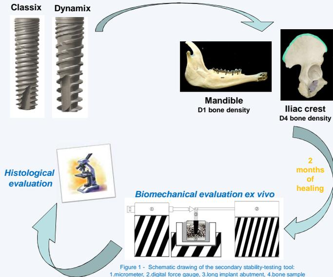
Figure 1 - Schematic drawing of the secondary stability-testing tool: 1.micrometer, 2.digital force gauge, 3.long implant abutment, 4.bone sample with the implant in place
